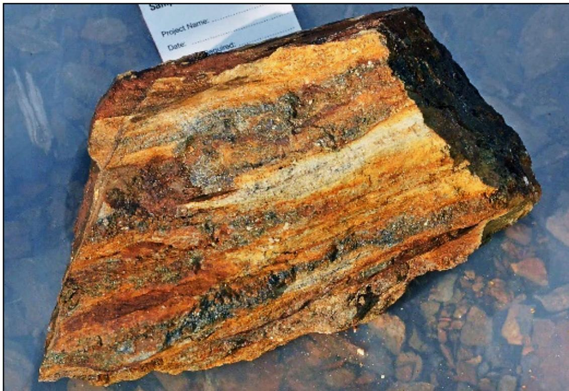
*Figure 3. Zinc (Fe-sphalerite) mineralization in quartz-sericite-pyrite schist collected by Project QP from the main trench in the Relf Lake Zone.*
