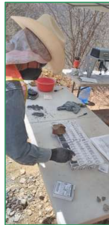
Chip logging with portable XRF in background
